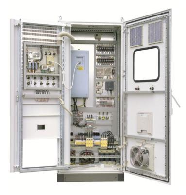
Pumping unit automatic control system cabinet ShSAU-NU is provided for automatic cost-effective control of electric drives in pumping units of different purposes, types and capacity with one or several pumps. Power limit of one pump is 1,5...160 kW, number of pumps is unlimited.
