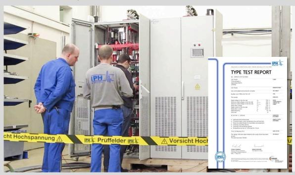
Rectifiers manufactured by PLUTON were successfully type-tested for the conformity to the International standards (IEC) and the European standards (EN) in test center IPH Institut (Berlin, Germany).
