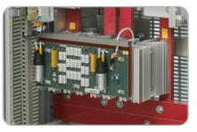
Galvanic insulation boards generate and provide information for analysis of the power diodes state diagnostics system with controller.
