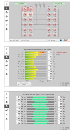
Information about state of the rectifier and its components is displayed on visualization panel, mobile devices (smartphone, tablet) or on the computer display via Web interface or special software.
