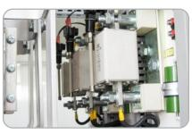
Protection of power semiconductor devices (diodes) against internal and external switching surges is implemented in rectifiers. Each diode is protected against internal switching surges with RC circuit, installed on the galvanic insulation board, and against external switching surges combined with RC circuits and variable resistor with fuses, installed on the switching surges protection panels.
